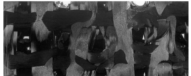
Figure 11 Edge notches due to debonding in the z -axis yarns.
